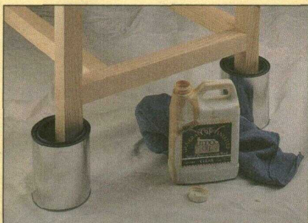
Water Repellent/Preservative. To seal the end grain in the legs, I let them soak in a water repellent/preservative.
